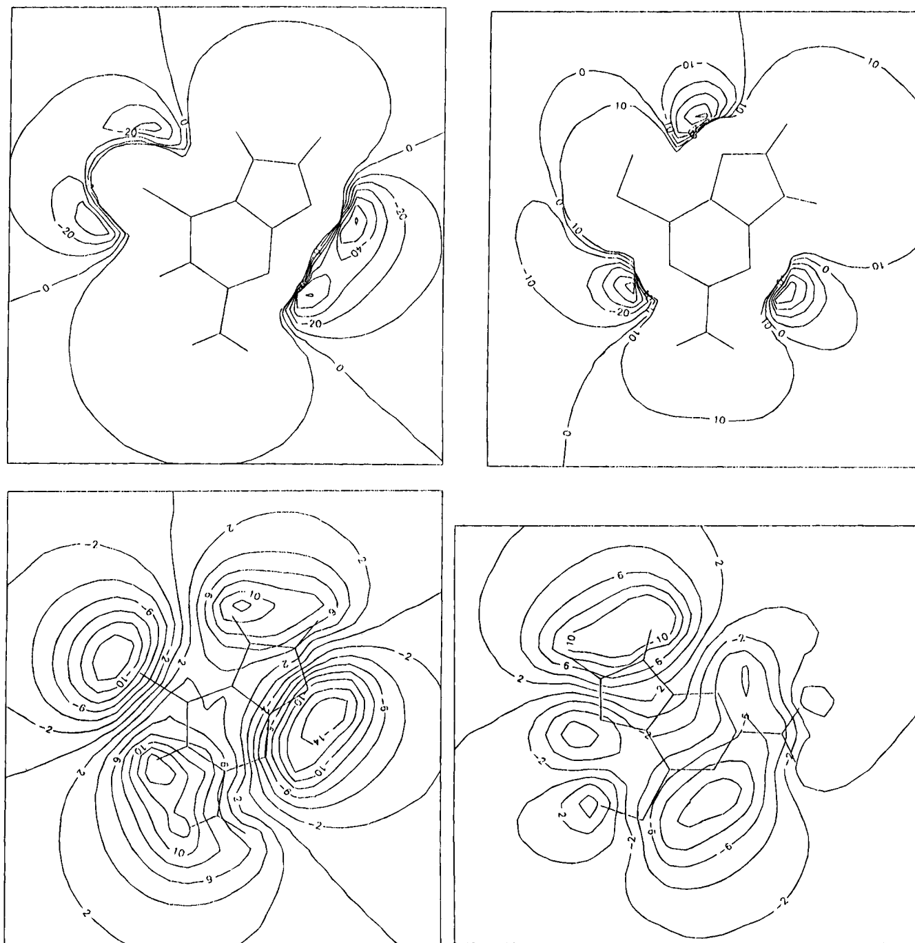
Figure 4. (A (Top left), A bis (top right)) molecular electrostatic potential (MEP) maps in the molecular plane of the S17 and SH9t tautomers of 6-thioguanine computed from 6-31G(d) gas phase wavefunctions. (B (Bottom left), B bis (bottom right)) MEP difference maps ( MEP_{aq} - MEP_{vac} ) in the molecular plane for the same tautomers. All the values are in kcal/mol.
